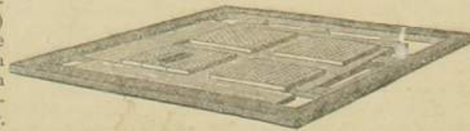
This process, which is called imposing , being completed, and the face of the types being levelled by a plainer and mallet, the form , as it is called, is proved,
